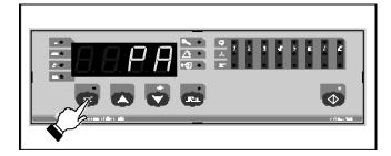
keep pushed at the same time for four seconds at least the up and the down key (passed four seconds the instrument displays /A1, the label of the first parameter of the second level).
