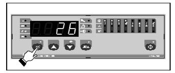
e) after the display push and release the set key (to the release of the set key the instrument displays the label Hr 7 again.
