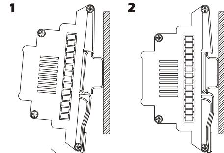
To remove C-PRO EXP MICRO, provide oneself with a screwdriver and operate as shown in the following drawing.
