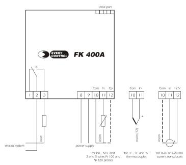
(12) provide the probe with a protection able to protect it against contacts with metal parts or use insulated probes.
