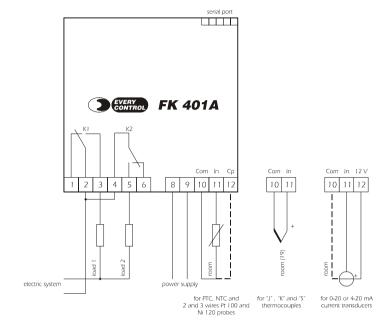
(19) provide the probe with a protection able to protect it against contacts with metal parts or use insulated probes.
