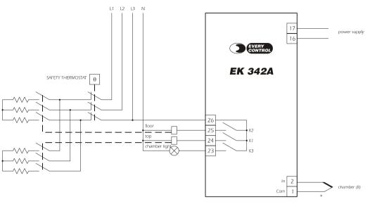
(8) provide the probe with a protection able to protect it against contacts with metal parts or use insulated probes.
