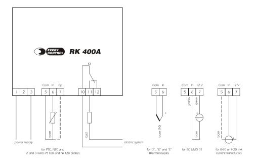
(10) provide the probe with a protection able to protect it against contacts with metal parts or use insulated probes.
