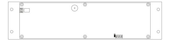
To disconnect the terminating resistors, position the jumper as illustrated in the following drawing.
