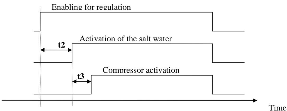
During normal functioning, if the absence of flow is detected for a time  $t_{FLO}$ , the alarm is activated that stops the pumps and the compressor.
