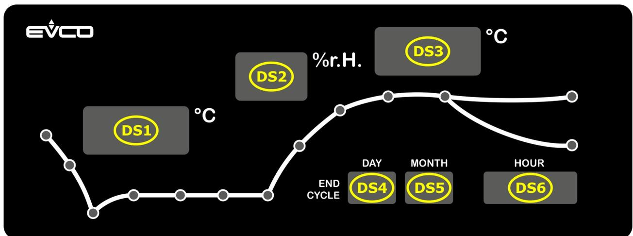
On system power on, the synoptic performs a lamp test with duration of 10 seconds.
