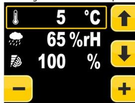
Pressing the UP/DOWN keys will change the e set-point to set. Pressing the +/- keys will change the value of the set-point selected. Pressing Home and Back are activated. Pressing STAND-BY is deactivated. Pressing START starts the cycle
