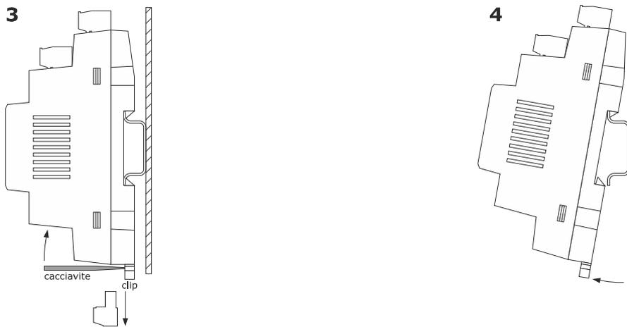
To re-install the device, first press the clip fully in.
